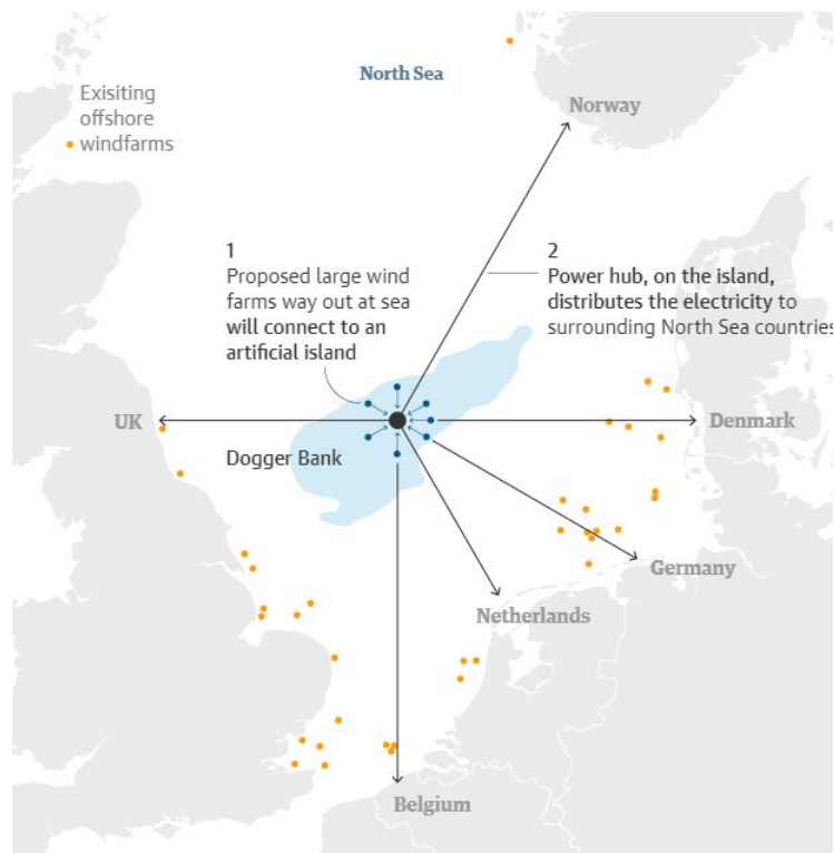
Figure 20: Dogger Bank where we can find high wind speed and shallow water, perfect for the implantation of an artificial island [26]
