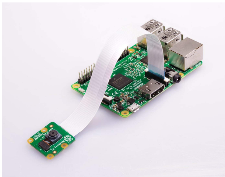
Figure 15: Pi Camera connected to the Raspberry
